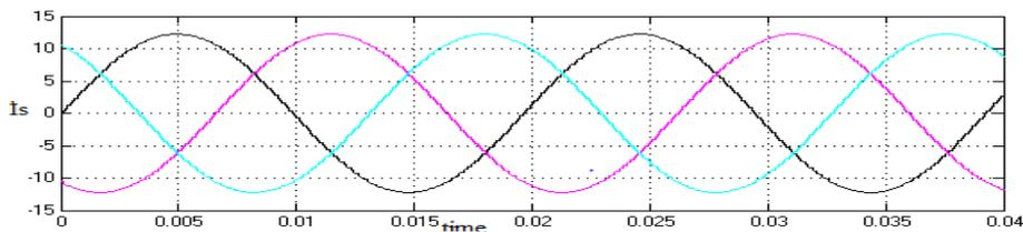
Figure 15: VSI Output Current Source.
