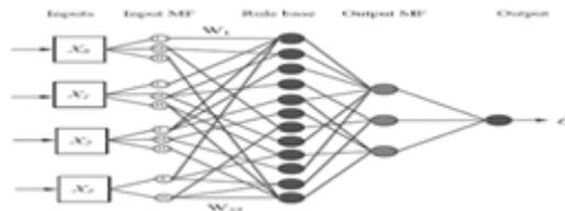
**Figure 7: General Structure for FNN Controller.**
