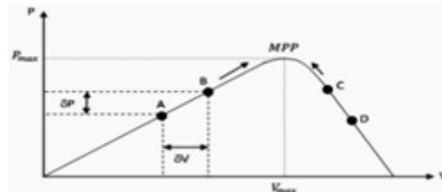
**Figure 2: Description of P&O Algorithm for MPPT.**
