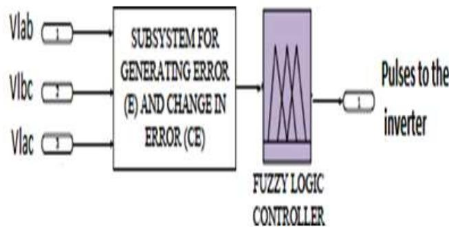
**Figure 5: Block Diagram of FLC Voltage Regulated Inverter.**
