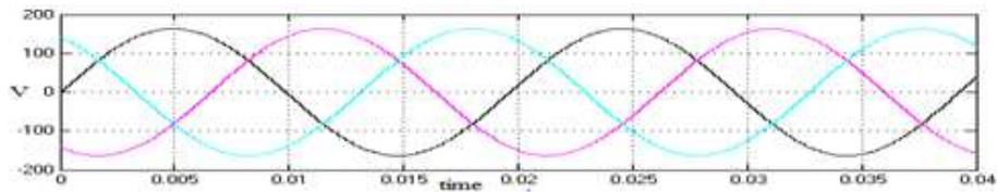
Figure 14: VSI Output Voltage Source.
