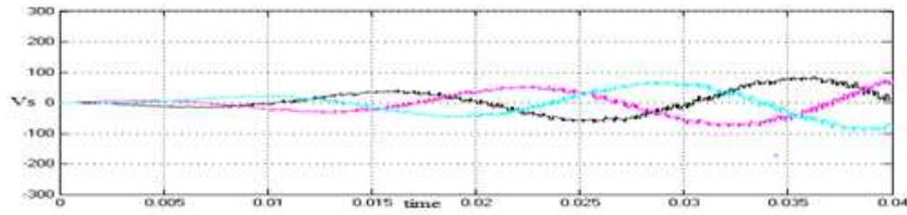
Figure 8: VSI Output Voltage Source.
